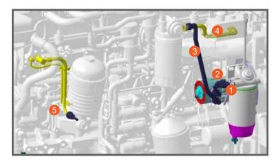
The inner diameter of the fuel hoses should be at least Ø10
